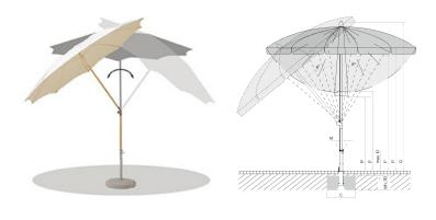
Loose cover max. 10 cm, concrete thickness min. 30 cm (pay attention to frost depth), Guarantee water drainage
