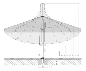
Loose cover max. 10 cm, concrete thickness min. 30 cm (pay attention to frost depth), guarantee water drainage, supply line electric.
